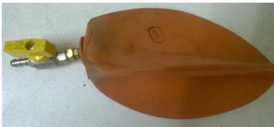
Figure 4.5: Bladder gas collection arrangement
